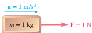
Fig. 1.2 A force of 1 newton applied to a body of mass 1 kg provides an acceleration of 1 \text{ m/s}^2 .
